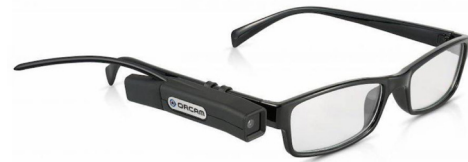
Image 5. Orcam - Text through audio feedback device for the visually impaired.
